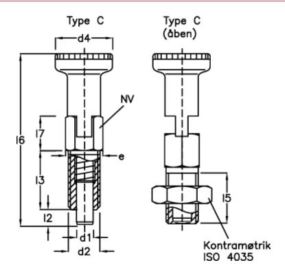
d1 = 6 I7 = 10.5 d2 = M10 NV = 10 d4 = 18 Spring pressure N bottom = 21 e = 11.5 Spring pressure N top = 5
